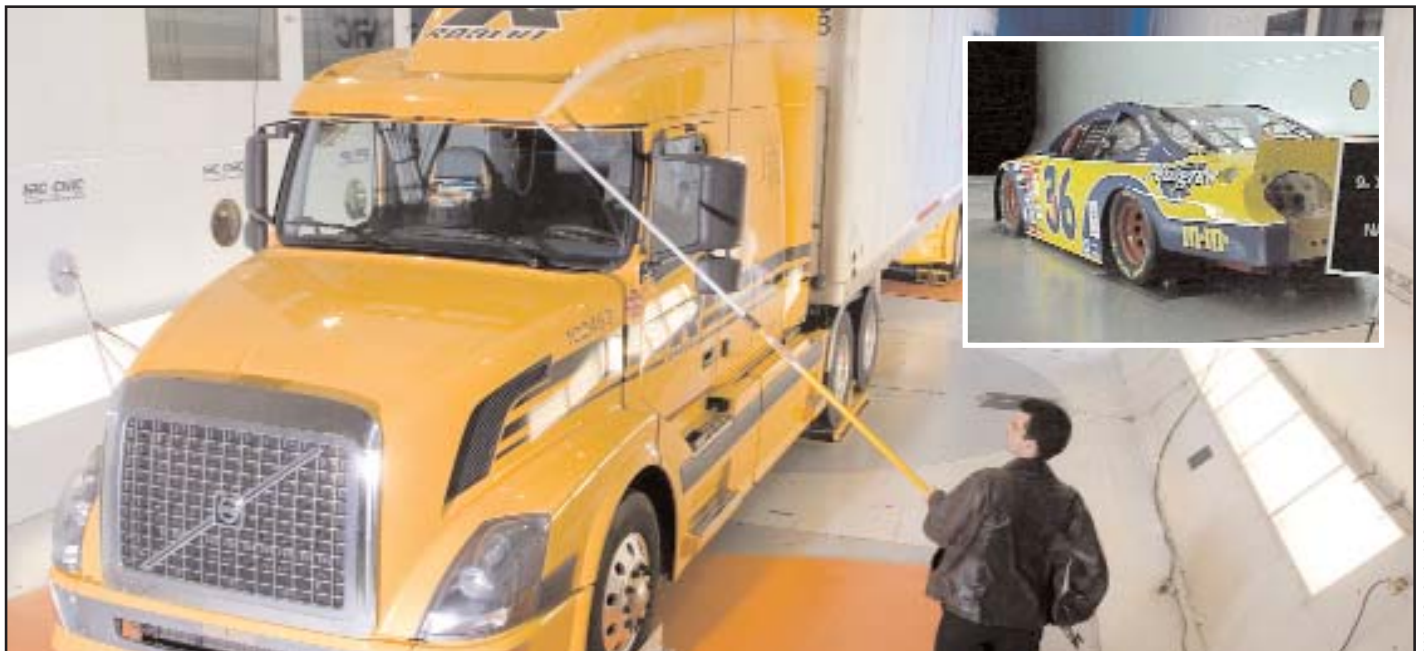
Wind tunnels test the aerodynamics of various shapes of vehicles, buildings and other subjects. Pictured above, a transport truck and a race car are being tested at NRC.
