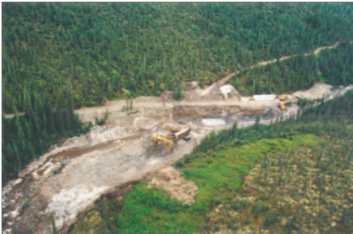
Figure 35. In 1996, Rivest Mining had a placer operation just above the canyon on Davidson Creek. Placer gold-bearing gravels were found on a low terrace on bedrock, and within a silty clay layer which may be McConnell glaciolacustrine sediment.
