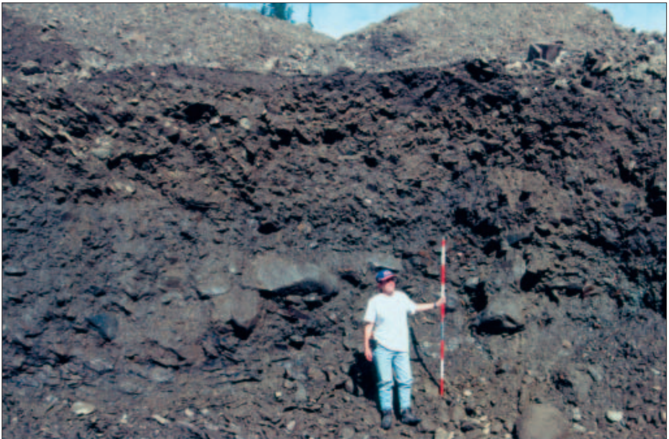
Figure 14. Facies 4 - Ggh, graded or graded stratified gravel, is distinguished by normal (fining upward) grading. It can be matrix or clast-supported with variably developed a- or b-axis imbrication. On Rudolph gulch this facies is the main pay gravel. This photo shows measured section RUD9701, where Facies 4 is interpreted to be a Holocene gulch gravel. Each division on the pole is 20 cm.
