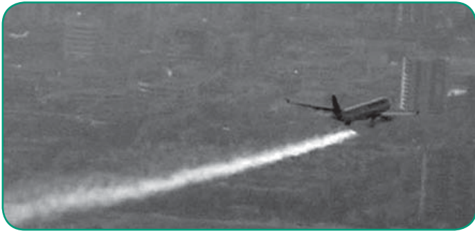
Visible fuel leak from the Airbus A330
