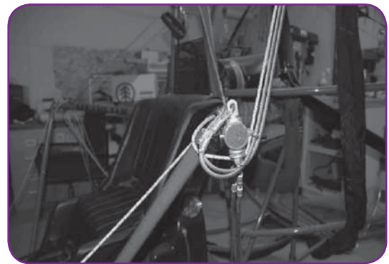
Figure 4. Photo of riser cables and steering line wrapped around the outrigger arm
