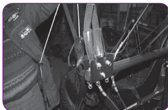
Figure 2. Close-up of newer design riser straps in the normal in-flight position
