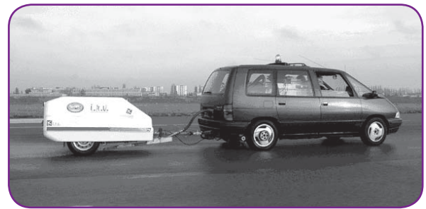
IRV used in the research program was this French-designed instrument de mesure automatique de glissance (IMAG)
