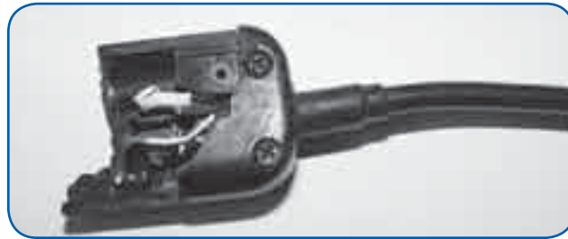
Figure 1. Fractured cord end fitting
