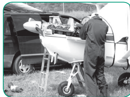
Field maintenance on a Cessna 172
