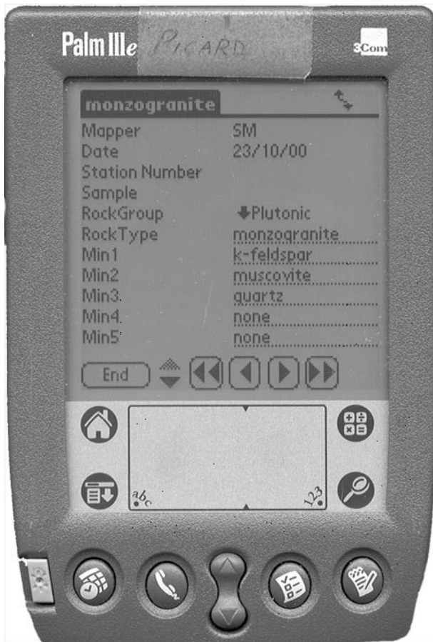
Figure 4. a) Rocks/Minerals thematic page of geological data-collection form (complete form available by scrolling up/down).
