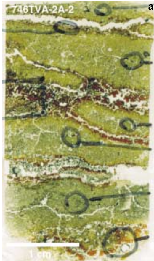
Figure 3a. Scanned image of thin section 74 GTVA. Marked circles indicate areas of study for the SEM and electron microprobe.
