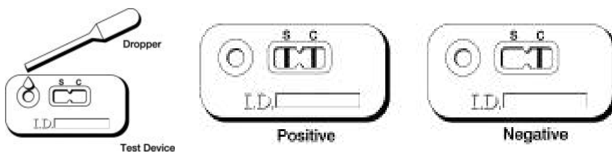
Figure 5- 11. BTA™ Test Strip testing procedure, Tetracore, LCC
