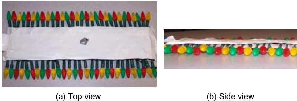
Figure 1. A mounted decorative light string prepared for testing.
