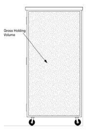
Measuring Interior Volume: Commercial hot food holding cabinet interior volume shall be calculated using straight-line segments following the gross interior dimensions of the appliance and using the following equation: interior height x interior width x interior depth. Interior volume shall not account for racks, air plenums or other interior parts.
