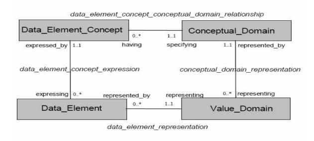
Figure 3 — High-level metamodel
