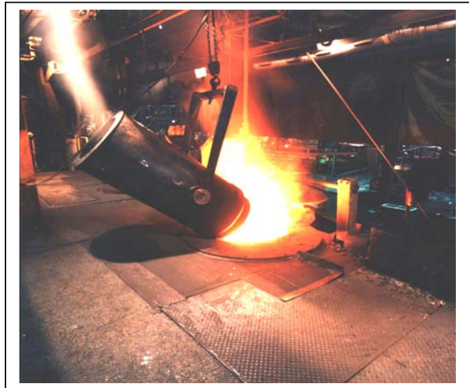
Preheated scrap being charged into the melting furnace.
