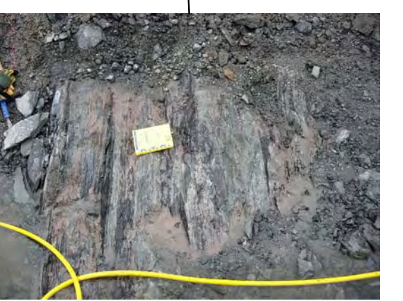
MASSIVE INTERBEDDED GREENISH MUDSTONE WITH BLACK SHALE (GREENISH MUDSTONE 10 TO 35cm THICK)
