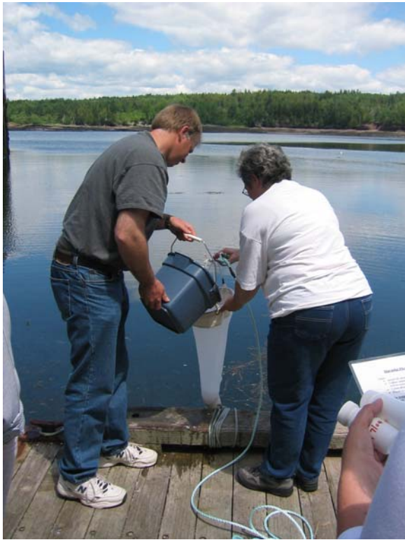
Demonstrating techniques for collecting surface water samples (left) and vertical tows (right) (7 July 2004).
