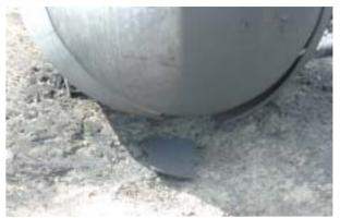
Figure 8 - Brittle Fracture of Tank 06-2
