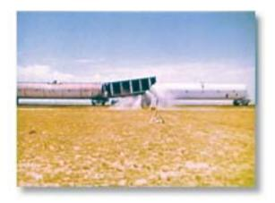
"Tests such as this one performed around 1980 led to the development of tank car head shields and shelf couplers. Further similar research and testing this year should lead to further enhancements."
