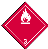
Class 3 Flammable liquids Flash point less than 61°C
