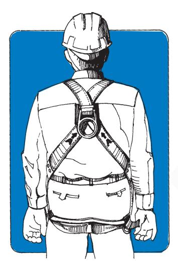
The arrows on the shoulder straps point to the only D-ring on the harness designed to safely arrest a fall.
