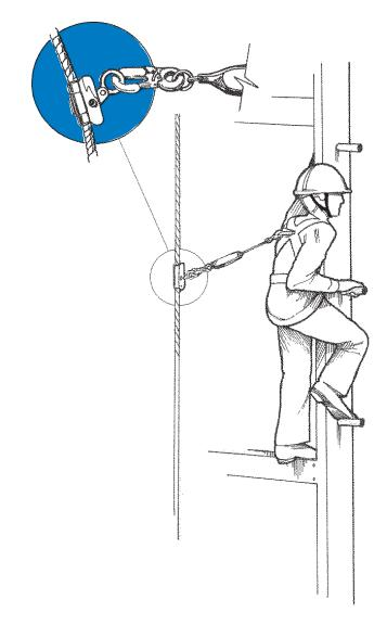
An automatic (or mobile) rope grab moves freely along the lifeline with you. If you fall, it locks automatically and stops you after a short distance. If you are using an automatic rope grab, it is recommended that you limit your lanyard to 0.6 m (2 ft.) in length.
