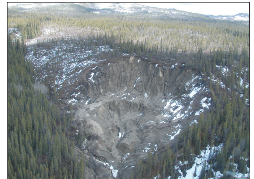
Large landslide that developed on a hillside 15 km southeast of Carmacks and travelled downstream over 4 km in a highly destructive debris flow, nearly blocking the North Klondike Highway.
