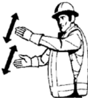
Slack the haulback. Hands in front of body using chopping motion.
