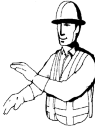
SLACK THE DROPLINE Cross arms in front and away from body flipping wrists
