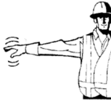
Slack mainline all off. Arm extended at side, flipping wrist.
