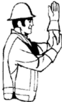
Ahead on strawline. Touch hand to bent elbow.
