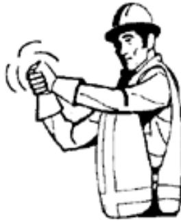
Hold dog drum or lock brake lever. Clasp one hand with the other.
