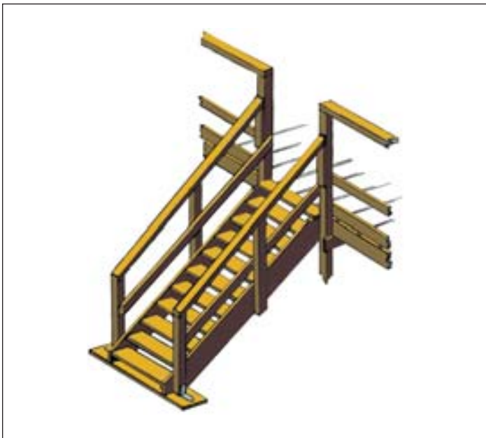
Temporary stairways with handrails.
