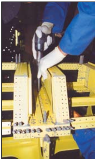
Pneumatic tools can transmit damaging levels of vibration to the hands
