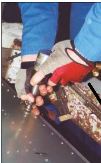
Anti-vibration gloves can reduce the risks associated with vibrating tools
