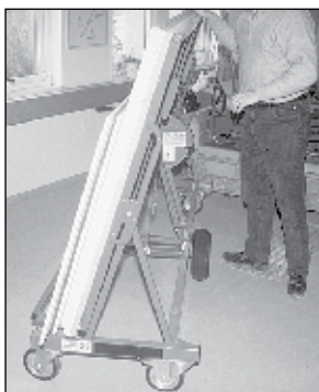
Adjustable tilt table can be used to transport heavy items
