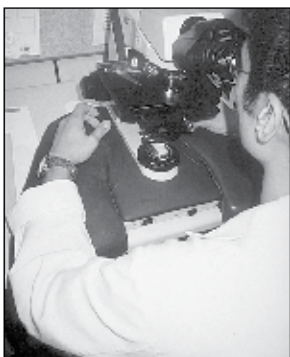
Armrest reduces contact stress on the arms while using the microscope
