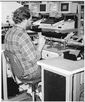
Create a cut-out work station to reduce the reach
