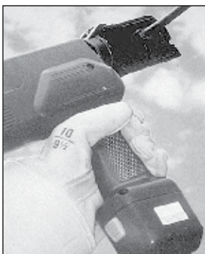
Gloves can reduce the contact stress from the handle grooves
