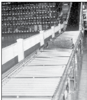
Conveyor can be used to shorten carry distances
