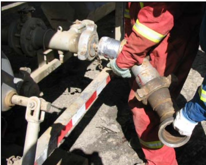
Photo 5: After the incident, workers indicate the position of the vent pipe assembly when the CO 2 operator attached it to the queen.
