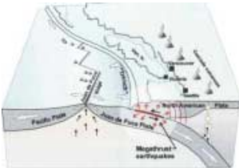
Cascadia Subduction Zone (CSZ) illustrating how the Juan de Fuca Plate subducts below the North America Plate. — Natural Resources Canada
