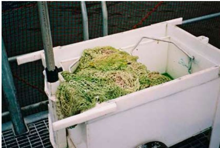
Escape recovery kit containing dedicated seine net and equipment to be used in the event of an escape. In the event of an incident this net and equipment is generally deployed inside a damaged containment net in an effort to prevent further loss of fish.
