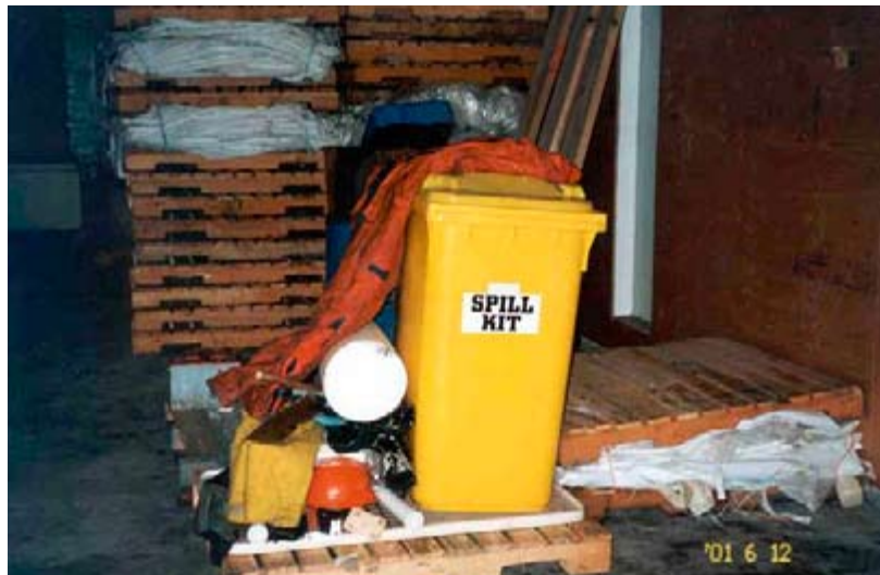
On-site spill kit and cleanup equipment.
