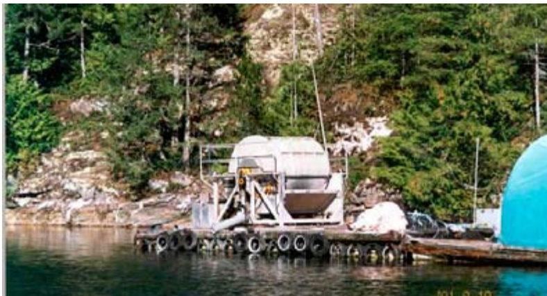
On-site net cleaning drum system.
