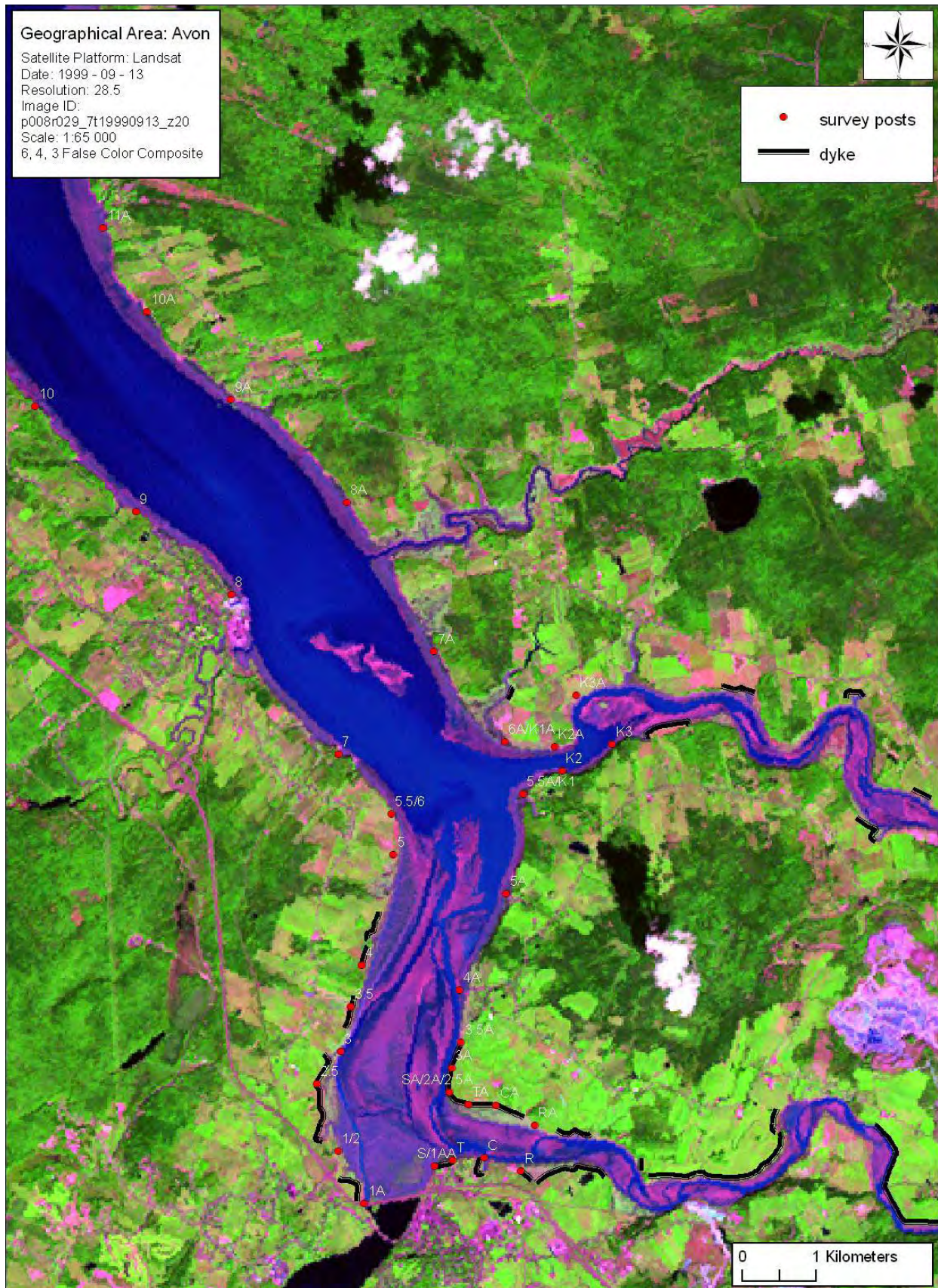
Figure 4.18: 1999 Landsat 7 bands 6,4,3 false color composite illustrating position of main channels and intertidal bedforms. Resolution of satellite is 28.5 m.
