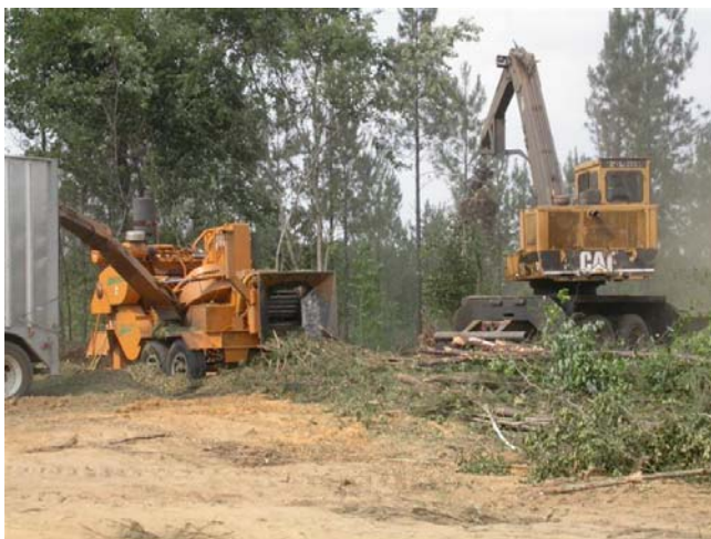
Figure 12: Full tree chipper situated on a landing, and loading directly into chip van.
