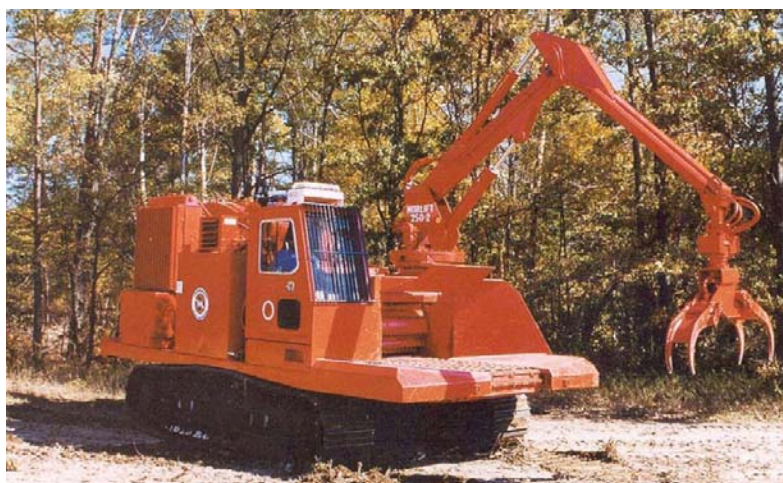
Figure 9: Track-mounted mobile chipper with integral grapple and straight-through processing path.
