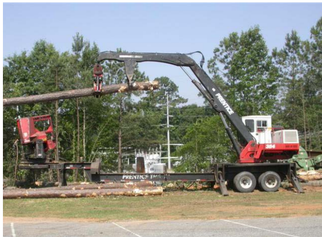
Figure 10: Trailer loaders include an integral delimeter/topping saw for processing sawlogs. The loader also feeds the chipper.
