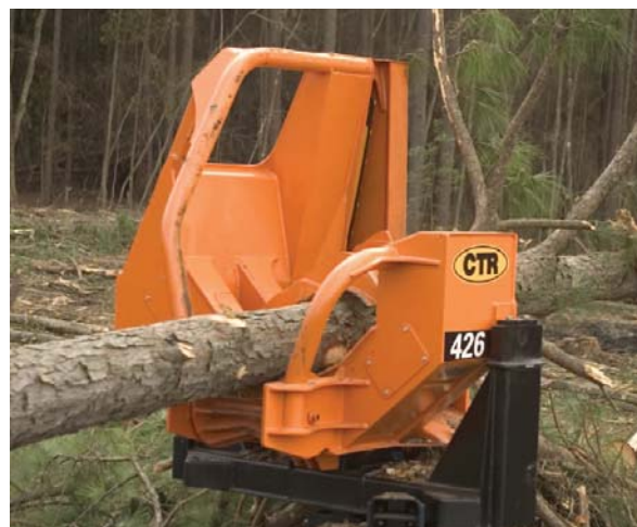
Figure 11: Pull-through delimeter and cut-off saw can be paired with conventional loader for processing sawlogs.
