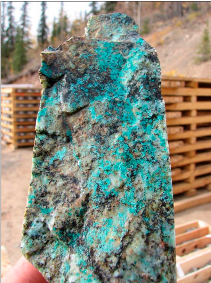
Figure 32. High-grade oxide copper (malachite) in core drilled in the No. 1 zone at the Carmacks Copper deposit.
