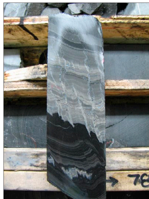
Figure 27. High-grade, laminated, low-iron sphalerite (grey) from the XY deposit at the Selwyn Project.
