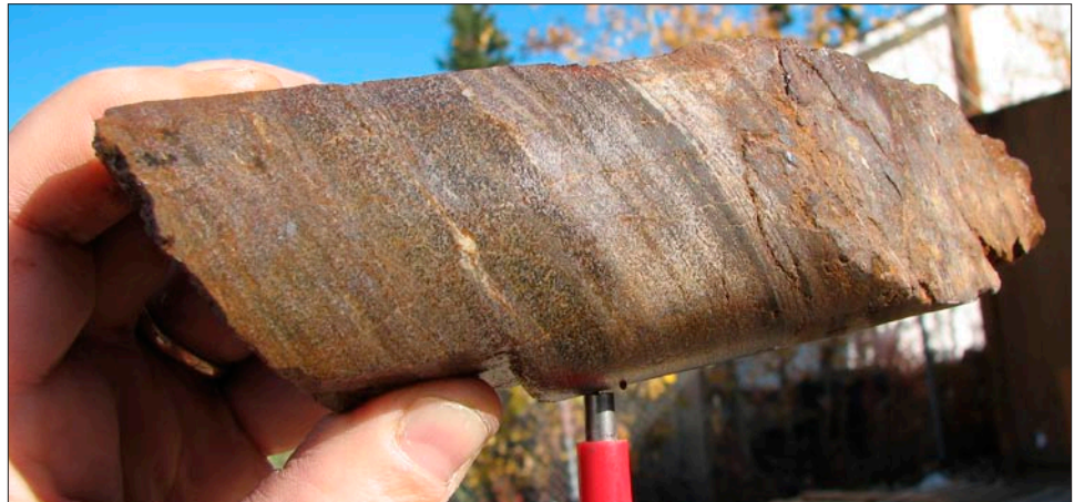
Figure 29. Magnetite in drill core from the Magnum project, a volcanic-hosted massive sulphide target in the Dawson mining district.
