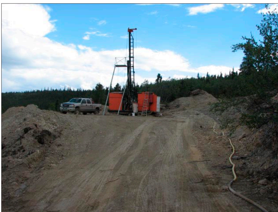
Figure 19. Diamond drilling on the Lone Star property in the Klondike.
