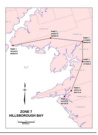
Points are referenced to the PEI Survey Reference System with all coordinates being expressed in metres. The projection (Double Stereographic), is referenced to the North American Datum of 1983 realized from the Canadian Spatial Reference System (NAD83(CSRS)). (EC766/05)
