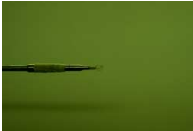
Figure 3: The Dantec tri-axial hot-wire probe mounted horizontally in the wind tunnel. Wind would be flowing from right to left during the measurements.
