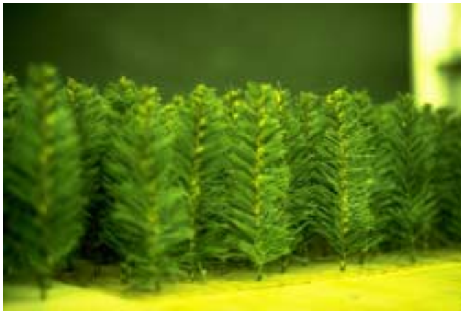
Figure 2: The 15 cm high model trees made from artificial Christmas tree branching used in the wind tunnel experiments.
