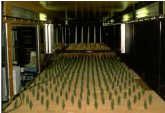
Figure 7: Looking upwind in the wind tunnel configured with a uniform model forest.
