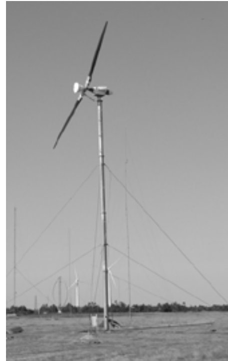
The Vergnet 60-kilowatt wind turbine is undergoing testing at the Atlantic Wind Test Site at North Cape.
