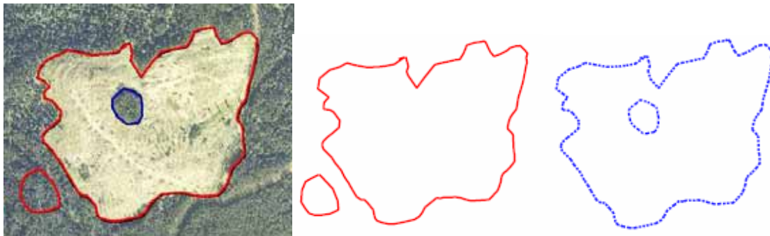
Figure 3.8.5-1: Left: Opening 1 - Clearcut with WTP's, 1 SU. Centre: Opening Boundary spatial data (red) - includes entire opening (productive, roads, WTPs, etc), and is a multipart polygon. Right: SU spatial data (blue) - Excludes WTPs and is a polygon with an internal whole.
