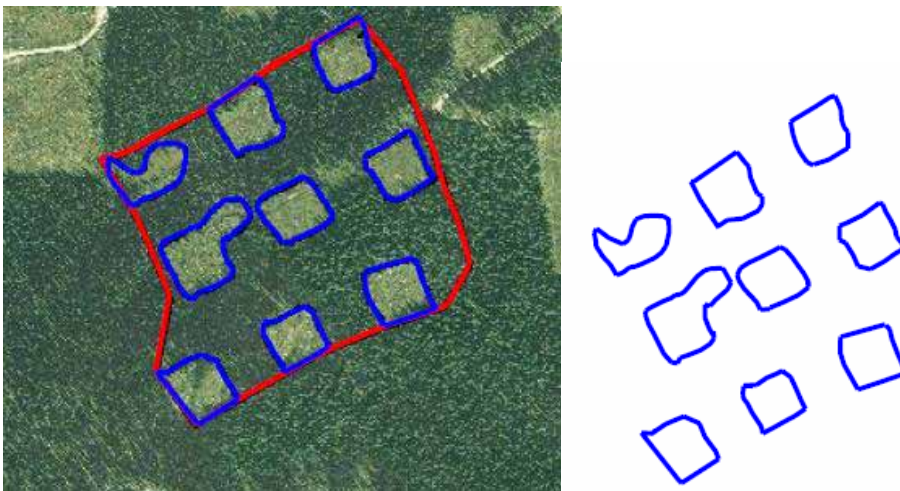
Figure 3.9.5-2: The opening (left) and the spatial data (right) for the disturbed area of the opening. This is a multipart polygon.
