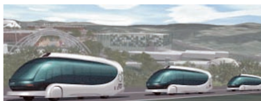
Intelligent Multimode Transit System (Toyota) combines the advantages of rail and bus transport. The buses run in automated platoons on dedicated roads, while on ordinary roads, each bus is manually driven.
