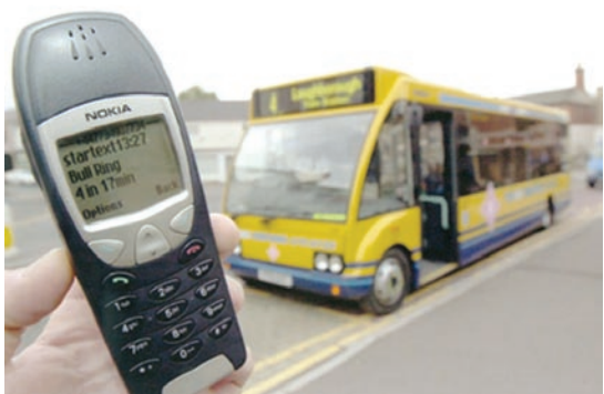
In Leicester, U.K., transit users can retrieve real times for all star trak buses on their cellular phones, by sending a six character bus stop code – found on all star trak routes – to an information number.
