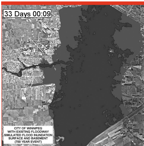
Impact of sewer and overland flooding on Winnipeg in the event of a 1-in-700 year flood with the existing floodway.
