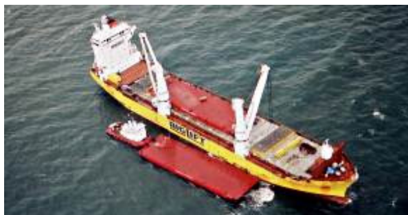
Barges being transferred from a heavy Lift ship in the Arctic in 2001 Image from Cooper Services web site
