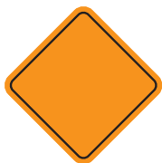
Orange diamond: Construction warning
