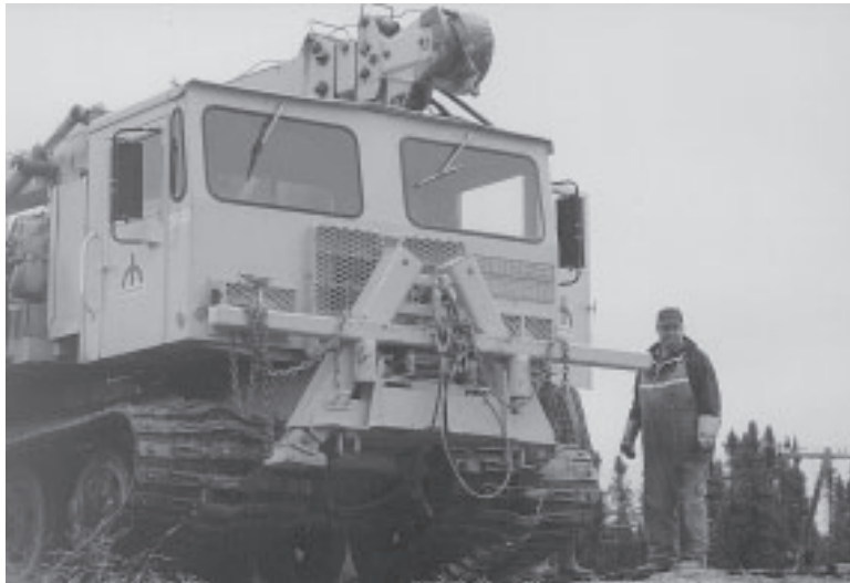
Use of wide track vehicles reduces impact on soil and vegetation.
