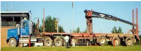
A truck with a legal lift axle at a New Brunswick scale.
