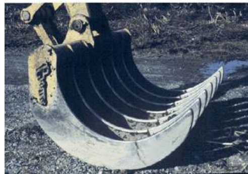
Figure 5. An excavator land clearing rake.
