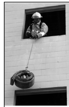
Figure 2: Then using a 19 mm (7/8") rope, hoist a hose roll weighing 18 kg (40 lbs) up 12.3 m (40'), then walk down the stairs to the...
