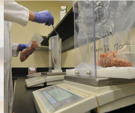
A Canadian Food Inspection Agency lab technician weighs a food sample for salmonella testing, which is an important step in matching a food source with reported cases of illness.
