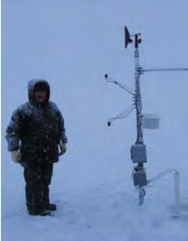
Figure 2. Ice monitoring station installed during the winter 2006-2007 near the Smith Island, Hudson Bay.
