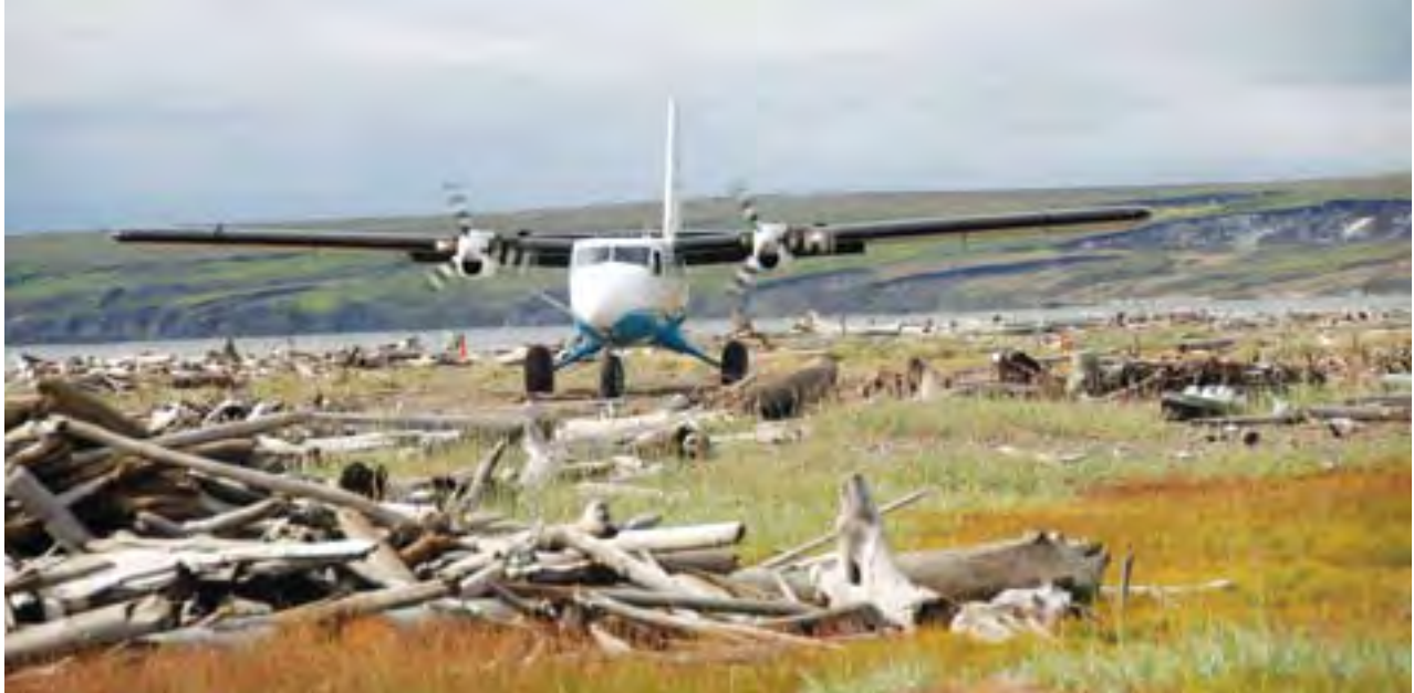
Figure 1. Twin Otter on the beach at Herschel Island, Yukon. Soft sandy storm deposits on the beach caused problems for aircraft landing in summer 2007. Note driftwood scattered near the strip and multi-cyclic retrogressive thaw-flow failures on the ice-rich slope in background. Photo: N. Couture, McGill University, 2007.
