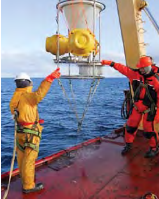
Figure 4. Retrieval of a sediment trap (vertical carbon fluxes) attached to a mooring cable. The sequential sampling cups are visible at the bottom. Photo: Keith Lévesque.
