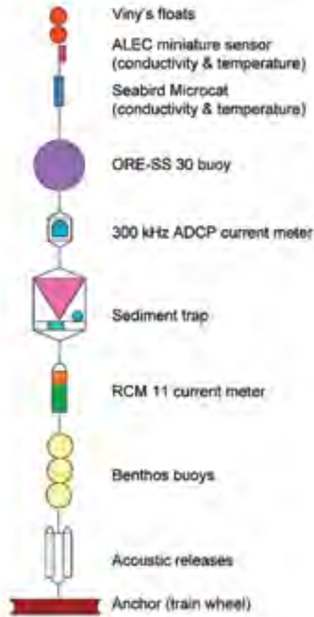
Figure 3. Schematics of a shallow mooring line, showing the sequence of various components on the vertical.
