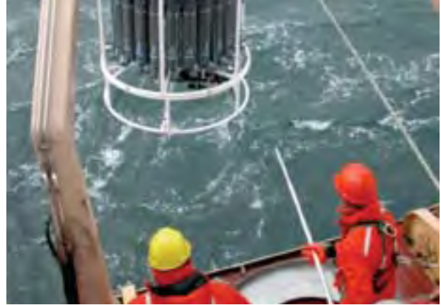
Figure 1. Deployment of the Rosette off the side of the CCGS Amundsen, showing the 24 sampling bottles and the site of sensors underneath. Photo: Martin Fortier.
