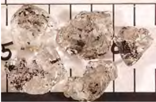
Figure 4. Mirabilite, a hydrous sodium sulphate salt ( \text{Na}_2\text{SO}_4 \cdot 10\text{H}_2\text{O} ), encountered in cores extracted from basin-floor sediments collected through the ice in a coastal breached lake near Sachs Harbour, Banks Island, NWT (Smith et al. 2006). Scale in centimetres. Photo: K. Jarrett, Geological Survey of Canada, 2006.
