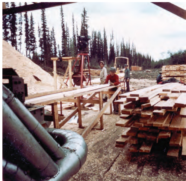
Feeding lumber into the planer at sawmill on Arctic Red River, NWT. Taken by Ted Grant, 1967.
