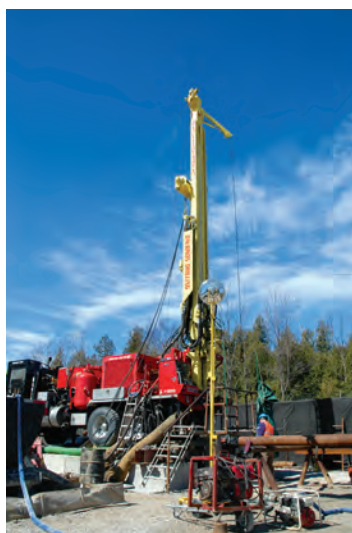
Deep borehole drilling provides site-specific data to characterize attributes of the geology beneath the Bruce nuclear site.
