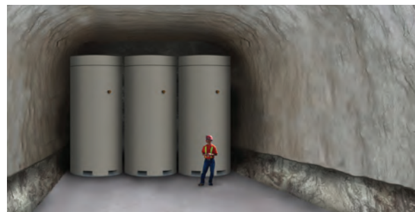
Intermediate level waste emplacement room.
