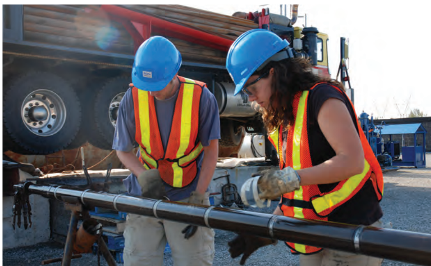
Deep borehole drilling provides site-specific data to characterize attributes of the geology beneath the Bruce nuclear site.
