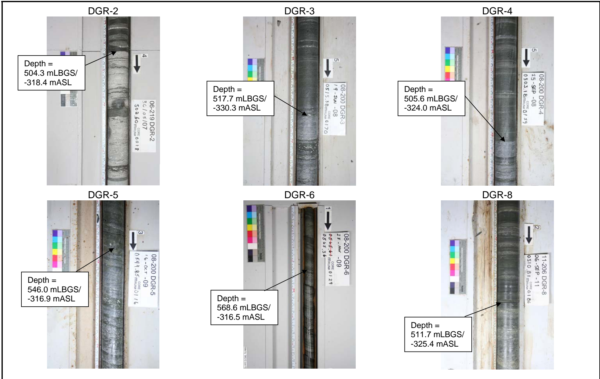
Queenston Formation - Limestone Marker Bed in DGR-2, DGR-3, DGR-4, DGR-5, DGR-6, and DGR-8
