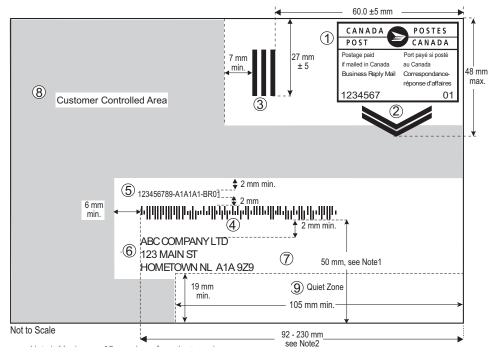
NOTE 1: Maximum: 35 mm down from the top edge; Minimum: 40 mm from the bottom edge.
