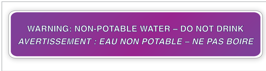
Figure 25 Typical marking for rainwater pressure piping
