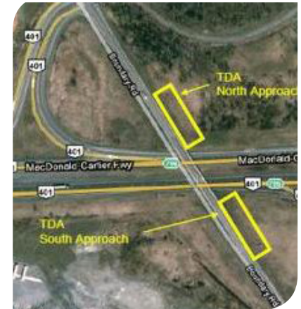
Embankment built with TDA on Highway 401 near Cornwall.
