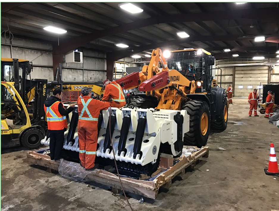
Figure 3: Mounting the Snow Lion equipment on a front loader
